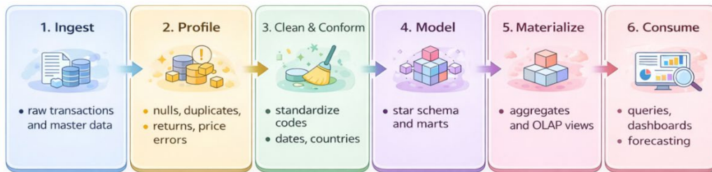
Figure 2: Processing pipeline from raw retail data to analytical consumption.
